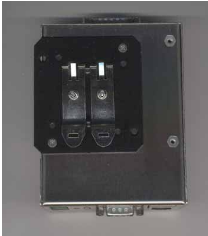
The bottom side with DIN rail installation part vertically.
